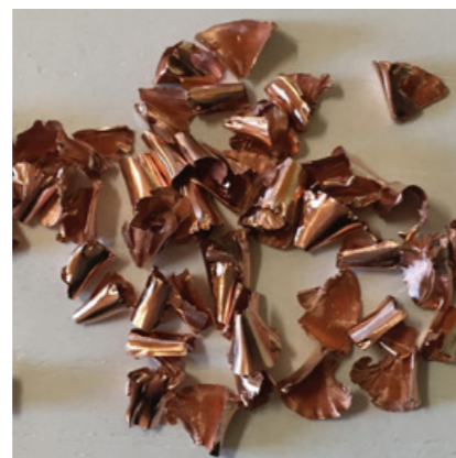
Picture of copper shavings removal 0,08 mm/sec with single blade cutters
