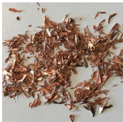
Picture of copper shavings removal 0.037 mm/sec with cutter RX Patent EP 2193003
